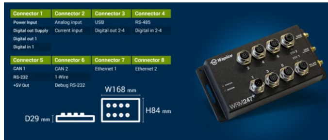
Figure 4: WRM 247+ device for remote management, measurement and control.
