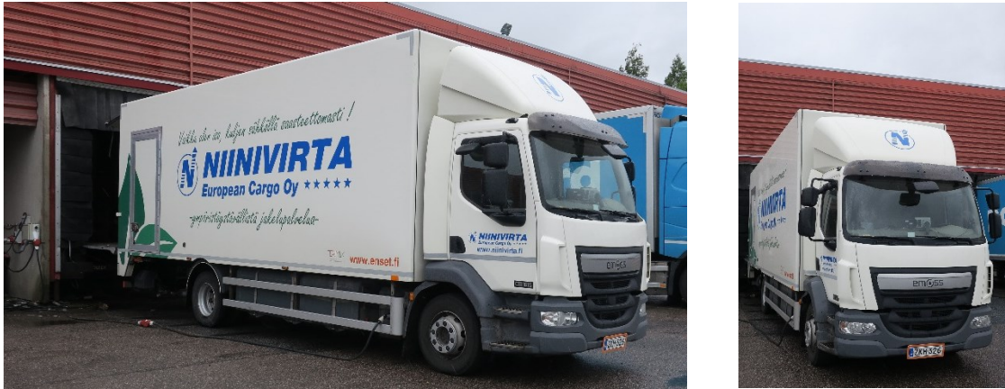
Figure 1: eTRUCK 16 ton electric truck in its present form connected to grid at terminal.
